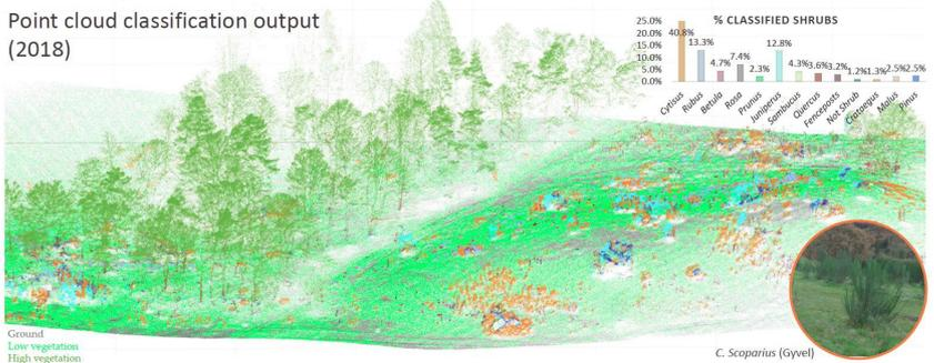
For example, based on the individual species in the 3D point cloud it is possible to estimate how much the volume has increased when flying over the area at different times. See [Madsen et al. Detecting shrub encroachment in seminatural grasslands using UAS LiDAR. Ecol Evol. 2020; 00: 1– 27.](#)
